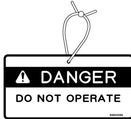
Operation prohibition during inspection and servicing. Hang this sign on the control lever during inspection and servicing not to allow any other worker to start the engine or operate the machine.
